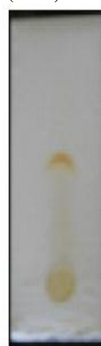
Fig 3b. T L C of Red cabbage Extract N-butanol, Acetic acid & Water (4:1:5)
